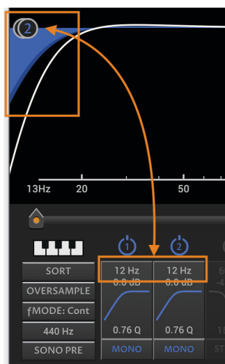
Figure 7: Two cascaded Sections with the “same” apparent f setting and differing actual frequencies
