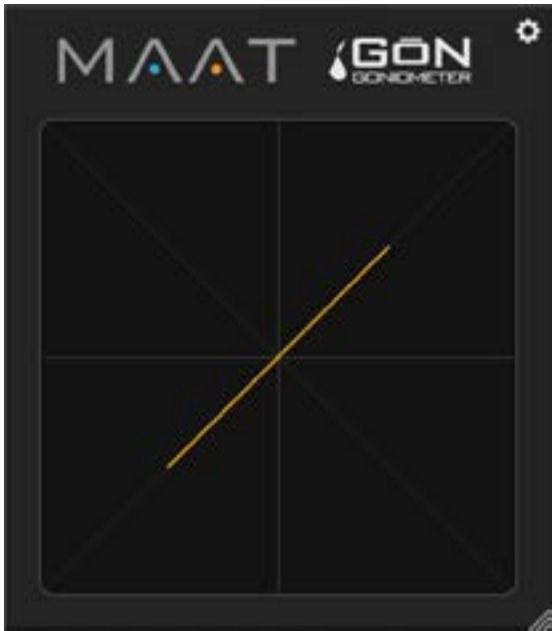
Figure 5 - A hard-panned mono input produces a variable length line at 45°
