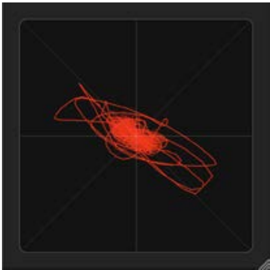
Figure 8 – The display “goes into the red” to indicate negative correlation
