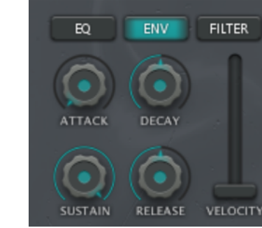
Envelope Panel Standard Attack, Decay, Sustain and Release controls along with a velocity sensitivity slider
